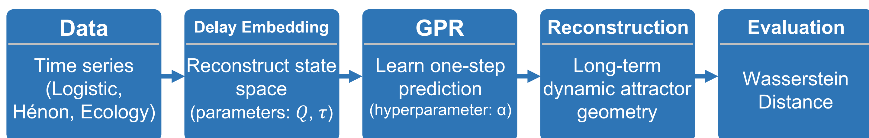
Figure 2. Workflow of the delay embedding and Gaussian Process Regression (GPR) framework used to reconstruct and evaluate system dynamics.
